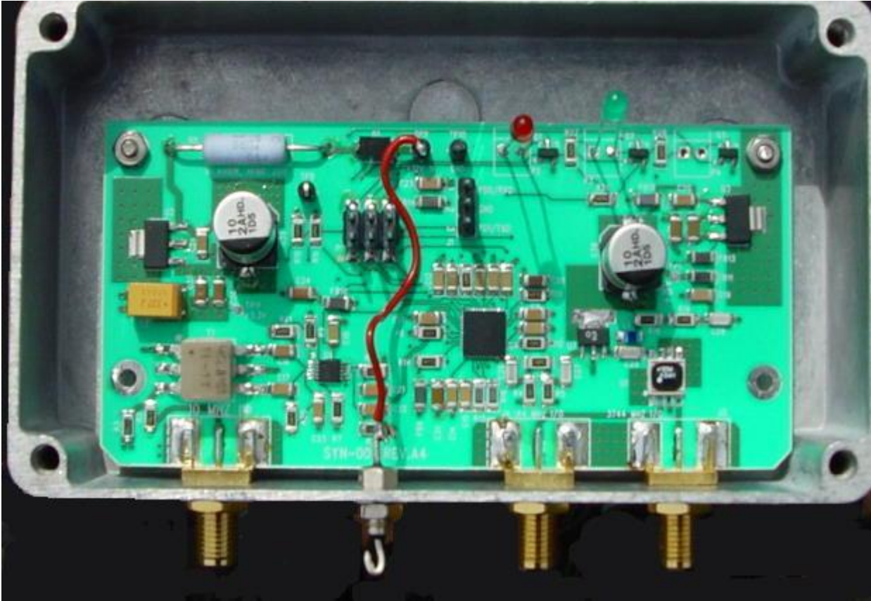
Figure 6 – Synthesizer / Mixer Board mounted in a Hammond box
