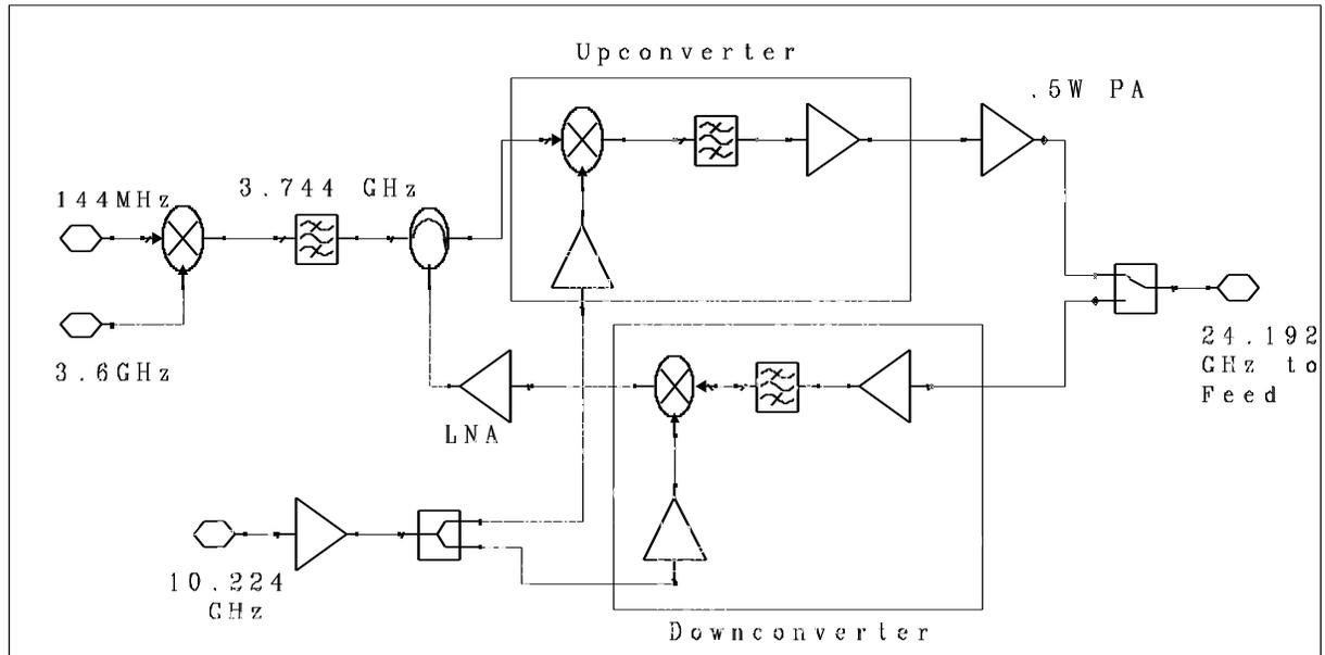
Figure 3 – 24 GHz RF section
