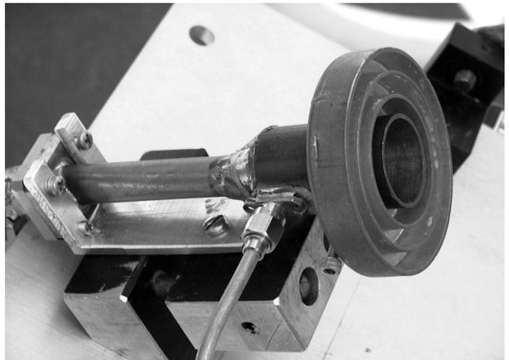
The feed horn sits on top of the RF plate that extends from the dish out past and under the focal point. The RF plate is ¼" aluminum about 36" long and 8" wide and is supported at the back of the dish and by two struts that extend from each side of the dish. The feed horn is mounted to an adjustable bracket that allows the fine-tuning of the position of the feed to the focal point.
