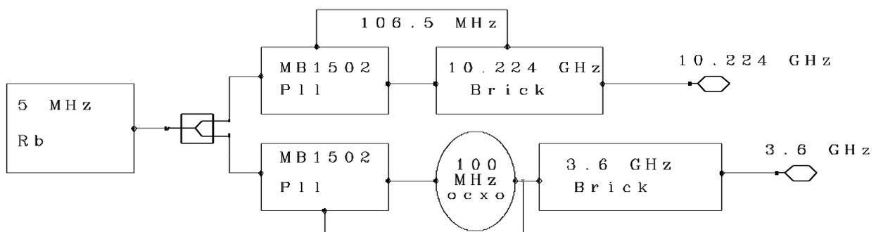
**Figure 1 - Local Oscillators and PLLs Block Diagram**
