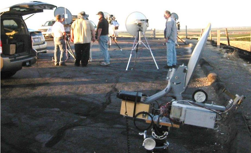
Mechanical Platform (Az-El pointing, level, tripod), T/R control, power supplies, battery
