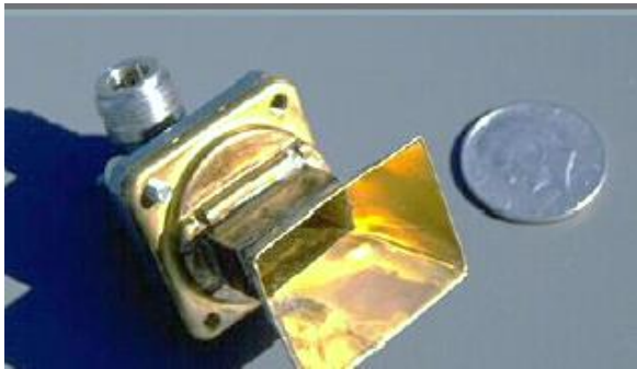
Template for 11.49 dBi horn for 10368 MHz
