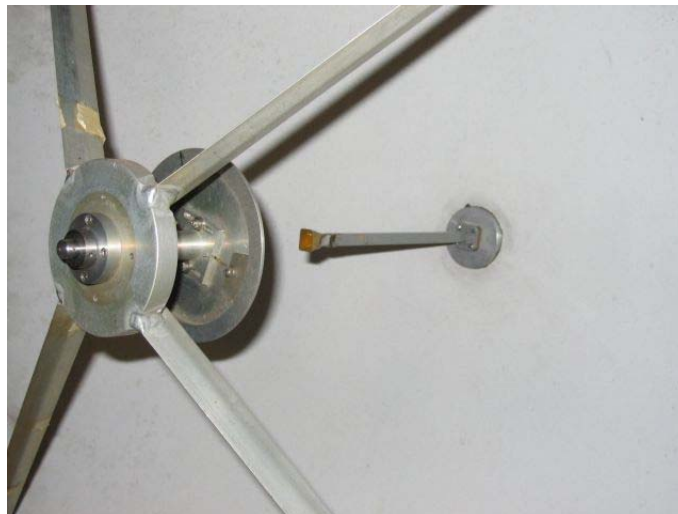
Figure 1 - 36" Cassegrain Dish Feed and Subreflector
