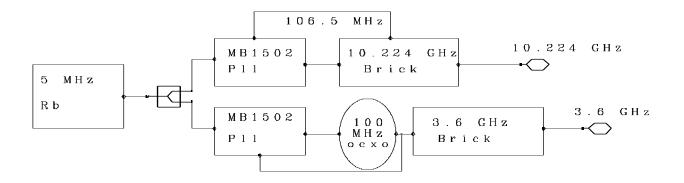
Figure 1 - Local Oscillators and PLLs Block Diagram
