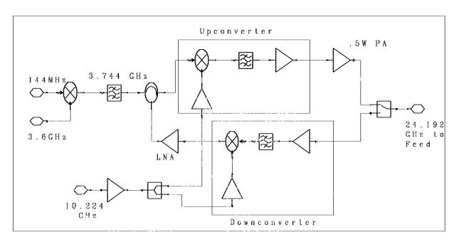
Figure 3 – 24 GHz RF section
