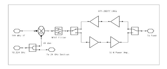
Figure 2 - 10 GHz RF Block Diagram
